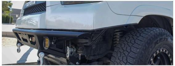
22) Raise the bumper back up to the cut edge. Install and tighten inner M10 bolts with washers.
