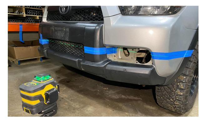
7) Undo any nuts / bolts / wiring attaching the stock plastic bumper to the vehicle and remove it. Or can leave it on the vehicle if desired, just make sure to not cut too deep behind the bumper and accidentally cut any wiring / fluid lines.
