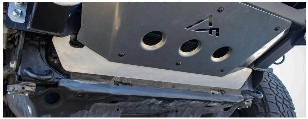
25) Install the lower aluminum cover using the 6x M8 flanged button bolts.
