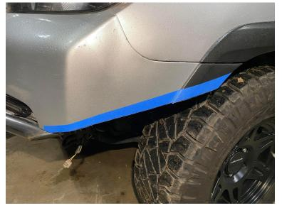
21) If desired, apply some weather stripping / edge guard to the cut edges of the stock bumper.
