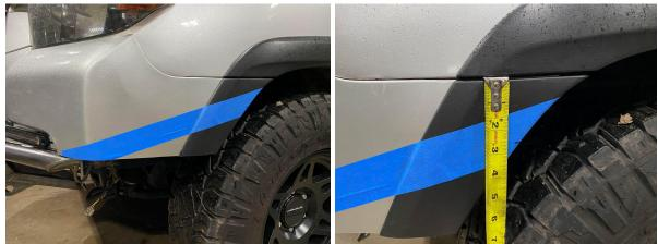
18) Use a flexible straight edge to draw a line from the outer wing of the bumper to the 2.5" mark on the edge of the wheel well.
