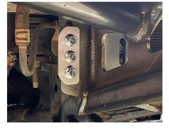
23) Install and tighten all 3x outer M10 bolts with aluminum washer plate per side.
